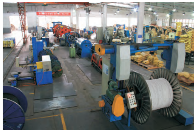
19盘成缆机 19 reel cabling machine
