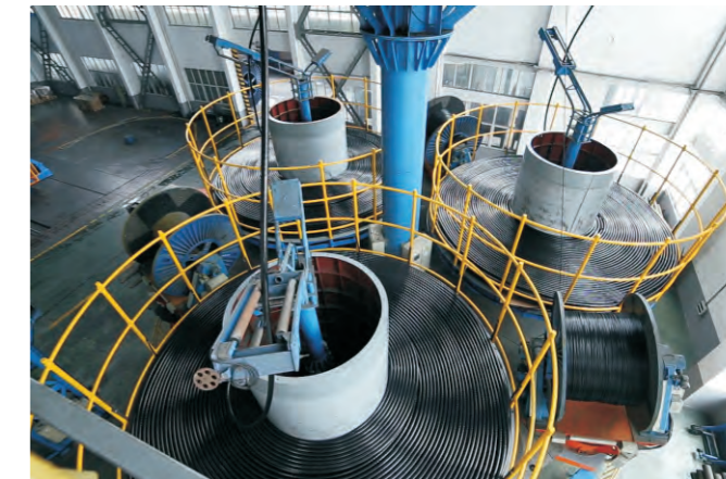
海缆立式成缆机 Subsea cable vertical cabling machine
