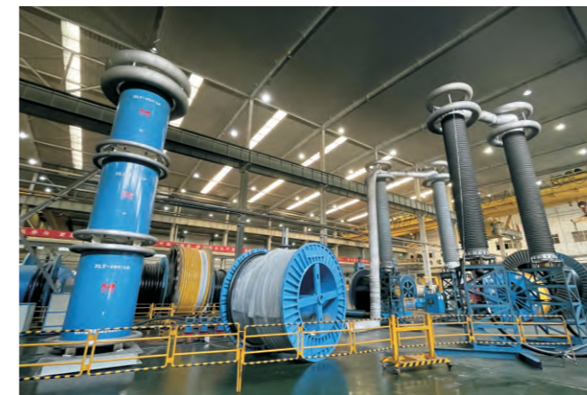
大长度1200kV直流耐压测试设备 Large length 1200kV DC voltage withstand test equipment
