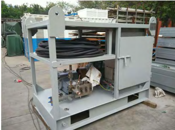
Hydraulic Test Pump Rated Capacity: 1.5m 3 /h&2.5m 3 /h Head of Delivery: 4000m
