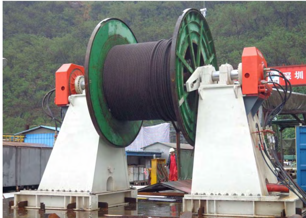
55 Te Spooler Max. Rotate speed (Installation): 6RPM Maximum Torque: 55KNm
