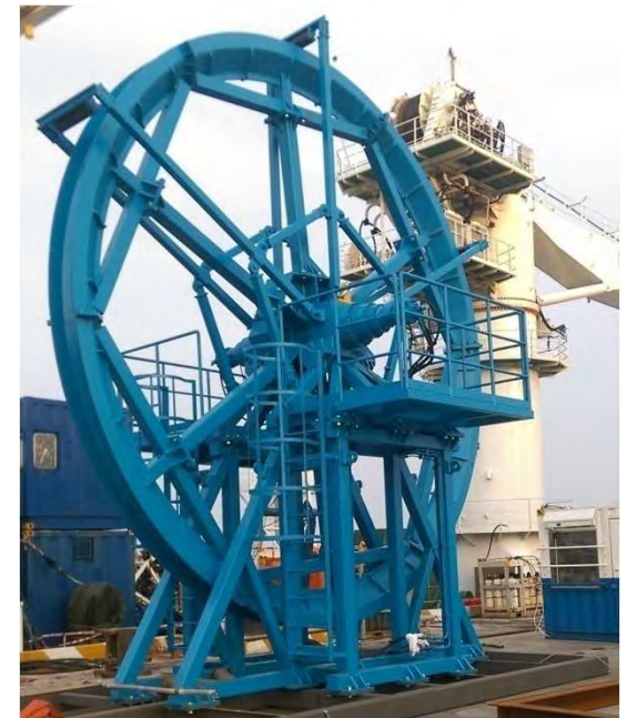
15Te Tensioner Speed (Installation): 1200m/h Product Diameter Range: 50~350mm
