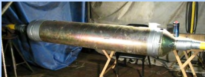
Submarine joints for power and OF cables
